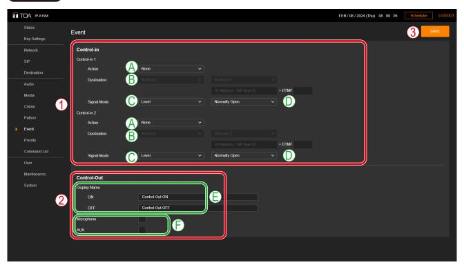
(1) Control-in Various event actions can be set for each control input, and can be executed by the input of a control signal from connected external equipment.
